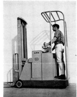
BEFORE MODIFICATION, A FORKLIFT SAFETY COVER offered little protection for operator Bob Tirnetta's (8245-3) head and back (left picture). After modification, the new cover and
